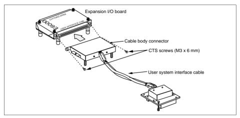
Figure 3 Connecting User System Interface Cable to Expansion I/O Board
